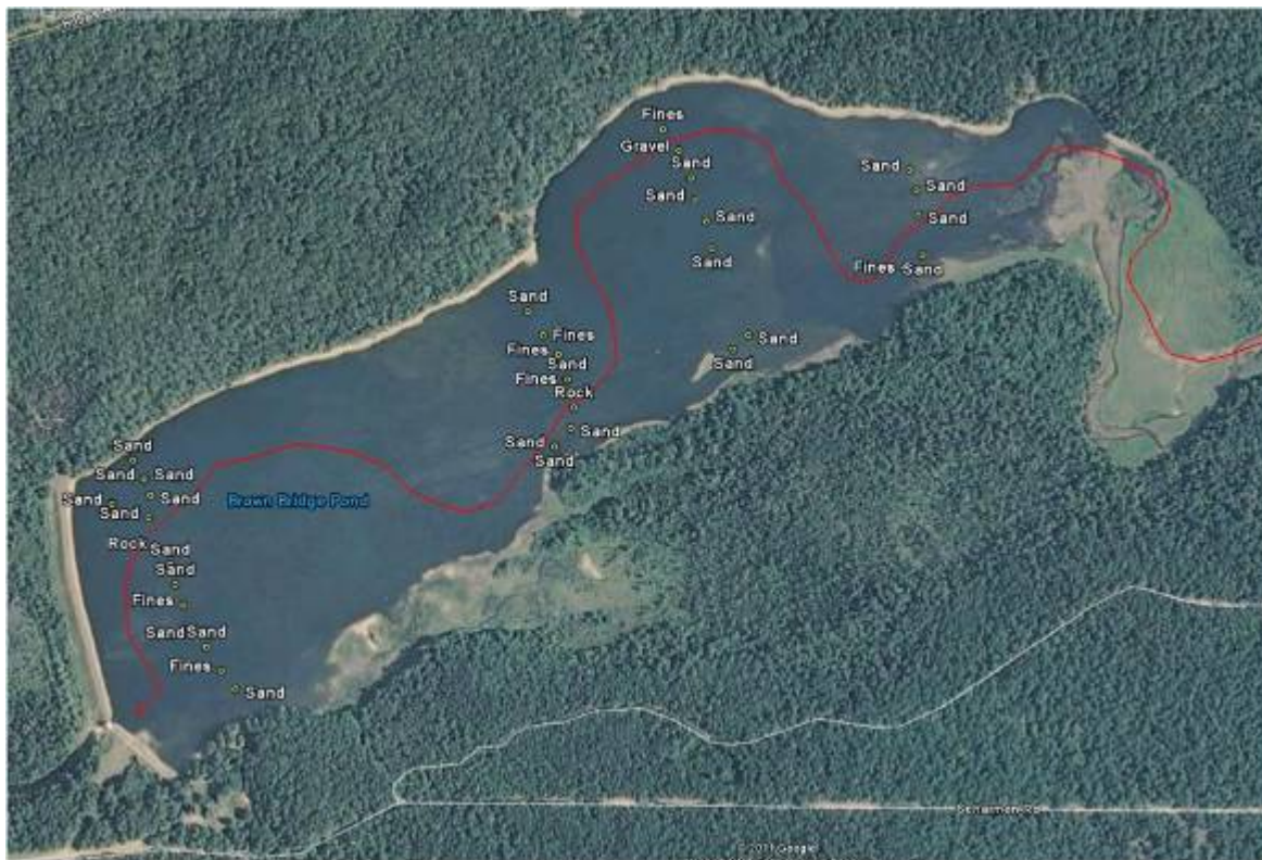
Figure 18. Bed Material Composition in the Lower Two-Thirds of the Brown Bridge Pond (Note: Red line indicates the approximate location of the pre-dam river channel based on bathymetric data.)
